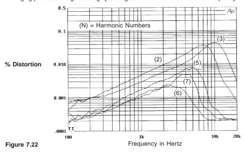
Showing the behaviour of individual harmonics 2nd to 6th Vs. frequency. In the AUT tested here, all follow the same pattern, but the order of the magnitudes does not follow the harmonic order - as co-revealed in the spectra.
