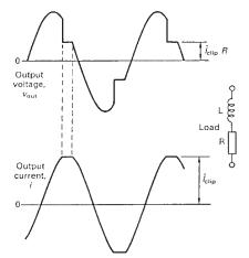
amplifier's output current clips into an inductive load (Figure 5.9). The feedback loop's restriction is dominantly caused in turn (at least in many conventional topologies) by a limit on the stage current  $I_e$ , that is available to charge an internal compensating or *lag compensation* capacitor,  $C_c$ :
