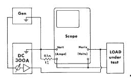
Note: Scope and amplifier grounds are not common. Vertical input reads (-) amperes vertically. If scope has an inverter, invert to read (+) A.
