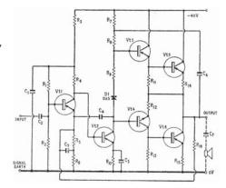
Today, the *Lin topology* is still the basis of many modern amplifiers, and also of classic, 3 stage, 'voltage-feedback' IC op-amps. For cheap, direct-coupled audio power, with high NFB, it seems elegant. Alas for quality audio, it is deeply flawed by asymmetries [10].
