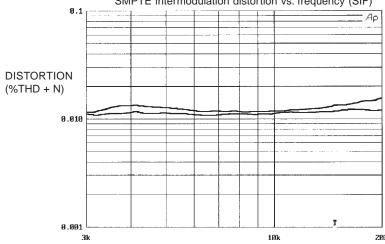
SMPTE intermodulation distortion swept against frequency. 3kHz is the minimum effective frequency. The almost flat curves are typical of linear, transformerless, electronic paths.
