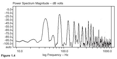
Fender Precision bass guitar's E-string, showing amplitude-frequency, i.e. spectral content, during the initial decay period after the Figure 1.2 transient. Reproduced from Stereophile magazine, with permission.
