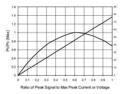
peak. On the right, % efficiency is scaled, and its straight-line slanting 'curve' is seen to rise in linear proportion to linear drive level, hence logarithmically in terms of dBs and approximate human perception of loudness.
