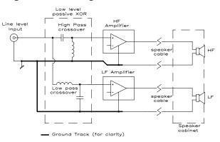
Otherwise, in ordinary 'mix and match' sound systems, one problem arising is that the crossover is physically divorced from the speaker, so careful connection is needed. Another, less daunting, is that any existing, passive high level crossover component values cannot be simply transferred, since they will have been 'tweaked' to best suit the vagaries of the drive-units' impedances.
