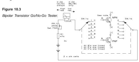
Several sockets to suit different pinouts are wired in parallel Two test sockets shown with NPN & PNP parts fitted In reality only one socket is used at once.
