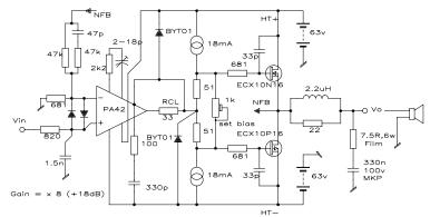
Figure 4.31 shows a test circuit used to demonstrate the PA42's application as an audio power-stage driver [31]. Clearly, the integration could be taken further. At the time of writing, the protection of audio power amplifier ICs against adverse loading still remains an issue, as *comprehensive protection is never included*, if not onboard, then in some separate protection IC.
