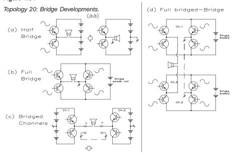
are also driven differentially, as indicated by the sinewave symbols – else there would be no effect. So a third perspective is that we have a balanced (or at least, differential) output also. One feature that is subtly different about Figure 4.34 (b) compared to (c) is that it has just one, floating, power supply. In other words, the bridging of a stereo amplifier with the usual independent, dual supplies is not necessarily the most elegant example of *bridgology*.
