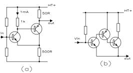
The *triple* (tripp'ull') is a mega-transistor built from three BJTs, and the natural progression of the Darlington. Figure 4.22 (a) shows the most obvious format – as still used by Crown. The sizes of the transistor symbols are a symbolic reminder that even more than with the Darlington, the transistors in a triple are cascaded in their current handling and capability, i.e. small, medium, then large.
