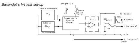
transient effects and protection circuit action, was published by Peter Baxandall [17]. Baxandall's circuit (Figure 5.30) drives the amplifier into hard but very brief clip, with  $50\mu S$  pulses on the back of a 20Hz sine wave. This enables the limits into reactive loads in particular, to be fully explored without stressing or destroying the amplifier, and with relatively little dissipation in the test load either.
