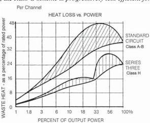
signal levels averaging >5dBvr, i.e. above 30% of full power. If the signal is compressed, clipped or bassy enough for this kind of condition to be prevalent, then the difference is a significant one: At 56% of full power (2.7dBvr), Carver quotes 65.7% whereas QSC's curve is indicating 76% with sine waves, and 82% with music drive. But with substantially uncompressed music and speech, i.e. purer live sound, the difference recedes.
