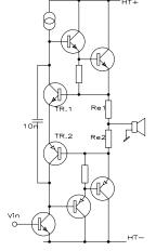
This same scheme also offers protection against short circuits, required with this push-pull output stage topology. Note that no such protection is required for the single-ended schemes that are biased by a constant current source – just so long as the current source controls itself against temperature.
