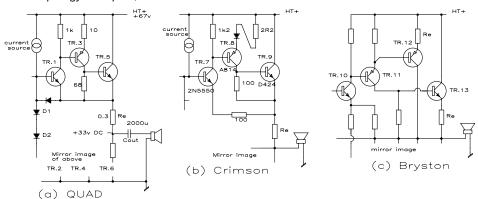
This particular topology has been instrumental ever since in BJT output stages of high sonic repute. One more of already several possible permutations (Figure 4.22 (c),(d),(e)), it is almost the same as Figure 4.21 (b) but with some major improvements, including being enclosed in a negative feedback loop, which not only linearises it, but prevents the latch up or 'sticking' with overdrive. Such 'dwell points' are quickly fatal to output devices, and are not good for sound either.
