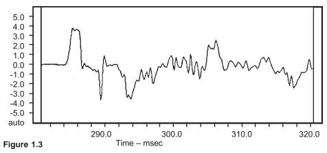
Fender Precision bass guitar's E-string, with the amplitude-time window magnified, out to 40mS (0.04 seconds). Shows overall asymmetry. The transient is the positive dwell point (at 288ms), followed by negative spiking (at about 289 mS). Reproduced from Stereophile magazine, with permission.
