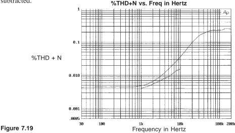
Classic %THD+N Vs. Freq. plots. The rise in the upper curve is partly arrested by the standard 80kHz bandwidth filtering and the AUT's own rolloff above 20kHz. The lower curve shows how the figure is not much lower with narrow band 400-22kHz filtering, with the sweep deliberately restricted to the meaningful 1kHz-10kHz area. The small difference shows that the '+N' is not the major component: the plot here is mainly harmonics.
