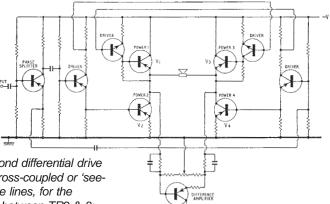
One reason to choose the bridge was the recognition that as with a push-pull stage (in the normal half-bridge), bridging cancels asymmetric differences – which create *even-order* harmonic distortion products. The foremost cause of such differences, at the time, was that between nominal *pnp* and *npn* 'complements'. Bridging excised these bugging little asymmetries. It seemed elegant at the time.
