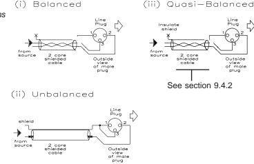
*Female* XLRs (sockets or receptacles) are almost universally used as the chassis mounted input on power amplifiers. There are at least two ways of wiring the incoming male cable plug, assuming one is used per channel.
