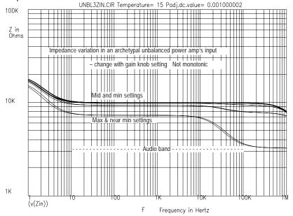
Figure 3.4 shows how the input impedance typically varies as the gain is adjusted. The change with each  $30^{\circ}$  rotation step is non-monotonic, so  $Z_{in}$  goes up then comes down, as you might expect. A  $10k\Omega$  log pot is assumed.
