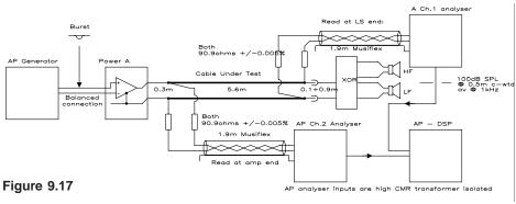
Test set-up to abstract error signals from a typical length of loudspeaker cable, under realistic conditions. Copyright Ben Duncan. All rights reserved
