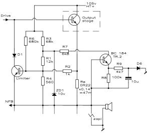
used, comprises seven paralleled power transistors, the effective value of  $R_e$  is about  $47m\Omega$ , if each leg resistor is 0R33.
