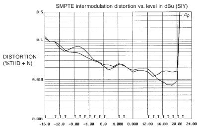
SMPTE intermodulation distortion swept against input level. This often manifests the 'V' shape for the same reason as dynamic harmonic distortion plots - the distortion-to-noise ratio, made visible by the low %THD of the AUT (as here) having respectably high linearity. The Timeout markers (T) confirm that the measured data was largely noise. The minimum may be taken to be the rated figure, i.e. about 0.01% SMPTE @ 1dB below clip.
