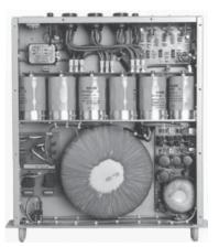
ensure for example that the HT supplies are not fired-up until the DC power plugs are all engaged, to avoid arcing damage to the contacts. A second case contained the similary seriously re-engineered audio stages.
