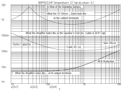
ability is degraded to, after is has traversed a given speaker cable and passed through an ideal  $10{,}000\mu F$  series capacitor, as commonly fitted in many professional cabinets for belt'n'braces DC fault protection. The rise at 1kHz is due to cable resistance, while cable inductance and the series capacitance cause the high and low-end rises respectively above 100 milliohms.
