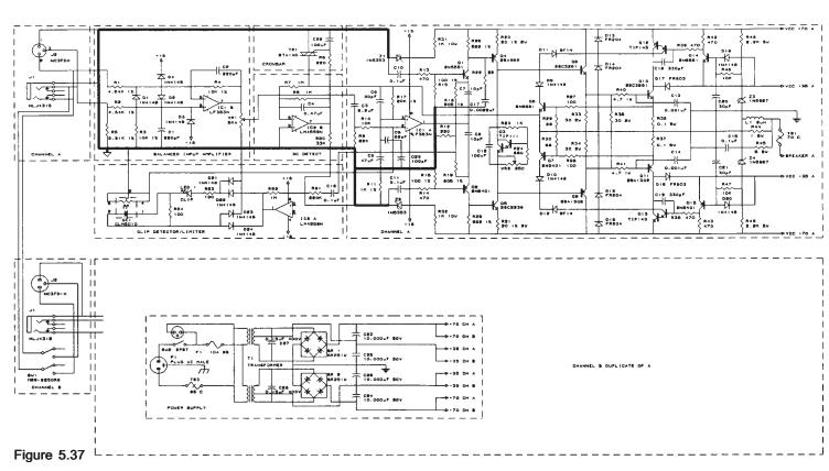
Circuitry of a rugged, high power, class G, PA amplifier, with BJT output. Protection and monitoring circuits include clip detector/limiter (bottom left); Input protection diodes (above); DC protection crowbar (above IC2B); and on the far right, centre, Zobel parts C13, R40; damped choke L1, R44 and thermal protection switch. Note also symmetrical circuitry based around an IC op-amp driver - see section 4.4.3. © Crest Inc.
