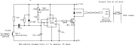
It is little recognised that *even when there is no music signal*, most solid-state power amplifiers can be stressed by (almost) *hard shorting* their output. This because in most designs, DC offset voltage provides a 'signal'. For example, if there is +50 mV DC at the output, and the output's source impedance is  $2 \text{m}\Omega$ , and the 'short' is  $35 \text{m}\Omega$  some way down the wire, then
