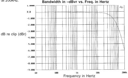
frequencies, this is unavoidable. But there should be no rise (+dB), and no peaks (+dB) nor dips (-dB) in the response, even where rolling-off. As in Figure 7.10.
