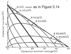
impedance reactances (+/ $-50j~\Omega$ ) that probe the high  $V_{ce}$  regions, where BJTs are most vulnerable to 2nd breakdown!
