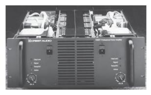
ratings, that individual hosepipe-sized power cords are fitted per pair of channels - hence the two power switch/breakers seen here. Notice the central tunnel cooling, and the general symmetry of the weight disposition, with end-on toroids up front, and reservoir capacitors behind. © Crest Audio Inc.
