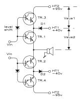
The outcome is cooler running, than if TR.3,4 with their +/-95v rails, were passing current all the time. In effect, switching is being used to improve efficiency within an analogue amplifier.
