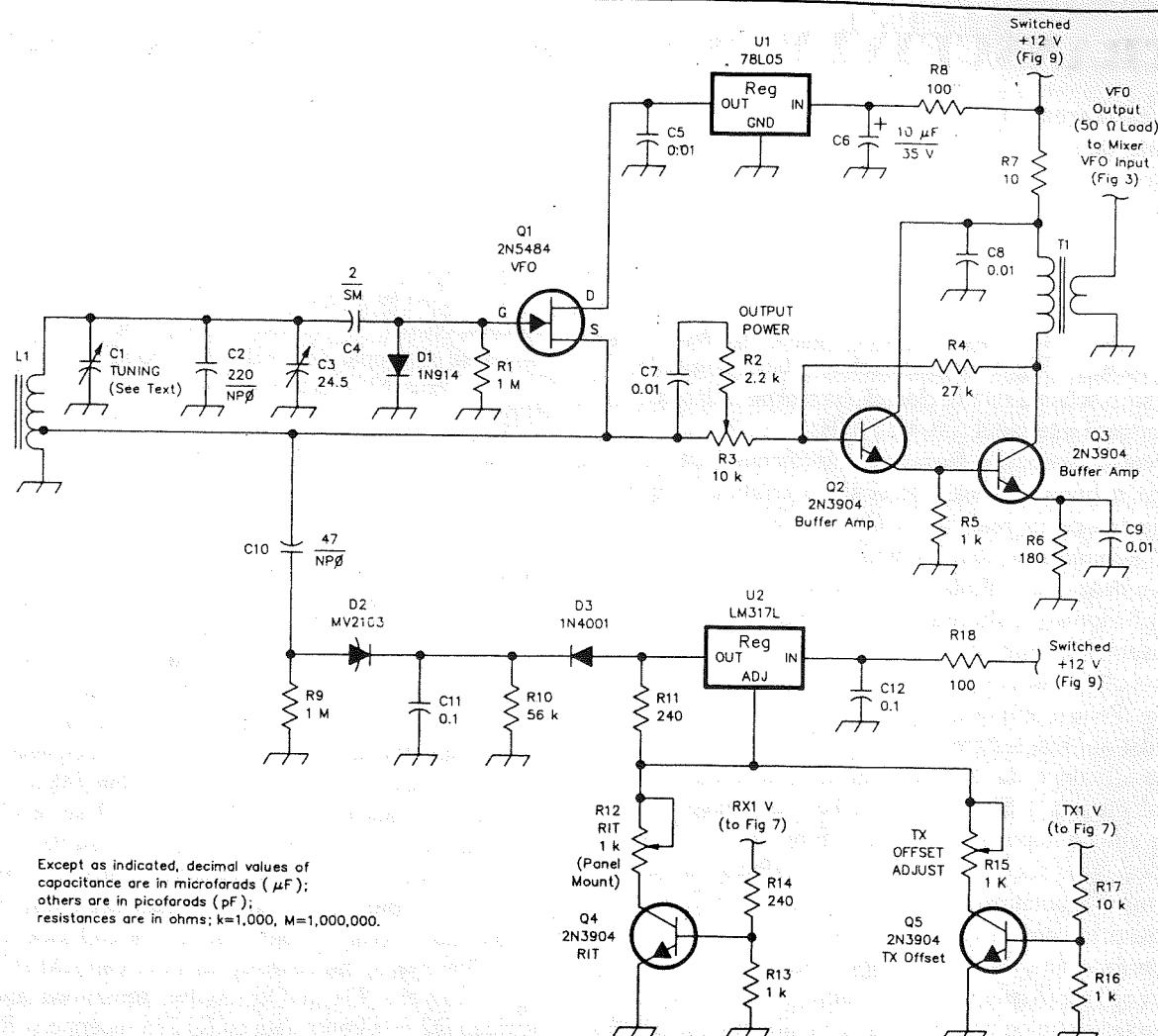
Except as indicated, decimal values of capacitance are in microfarads ( $\mu F$ ); others are in picofarads (pF); resistances are in ohms;  $k=1,000$ ,  $M=1,000,000$ .
