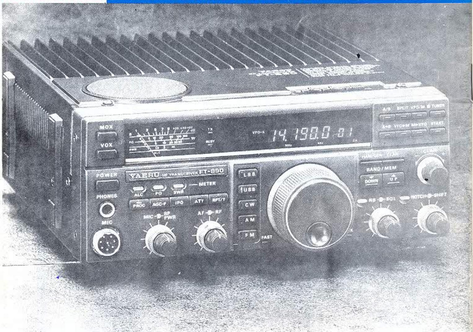
Blending the high performance digital frequency synthesis techniques from the FT-990 and FT-1000 with the convenience and affordability of the FT-757GX, the FT-890 adds a built-in (or optionally remote) automatic antenna tuner and a wealth of convenient functions. For compact base and mobile stations, the FT-890 sets the new performance standard.
