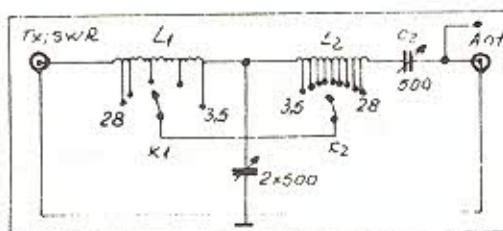
$L_1 = 8 \text{ sp. CuE } \phi 1.5, D = 40 \text{ mm}, l = 2 \text{ m}$
